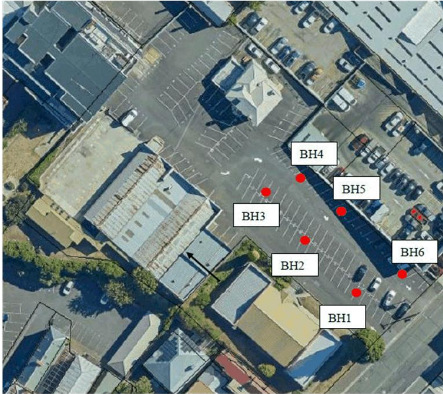
Figure 7.7 – Borehole locations January 2025. Geo-Environmental Solutions (p12).
