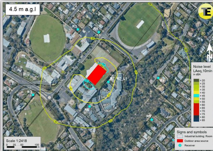
Figure A-2: Predicted noise emission contours, crowd and amplification noise, L_{Aeq,10min} , level 1.
