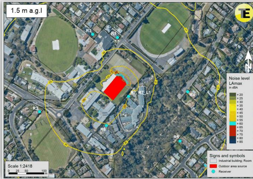
Figure A-3: Predicted noise emission contours, siren and ball impact noise , L_{Amax} .
