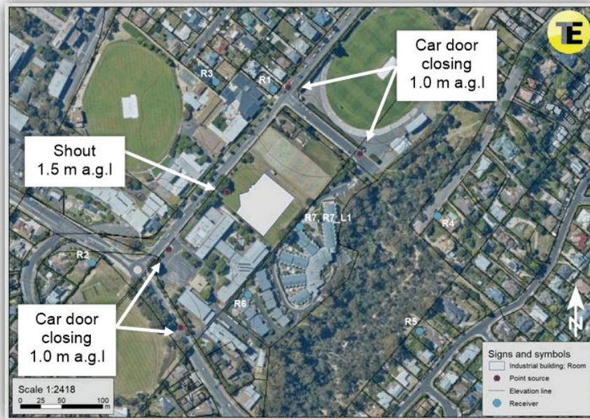
Figure 4-3: Environmental noise model plan view, departure noise, car door closing and shout.
