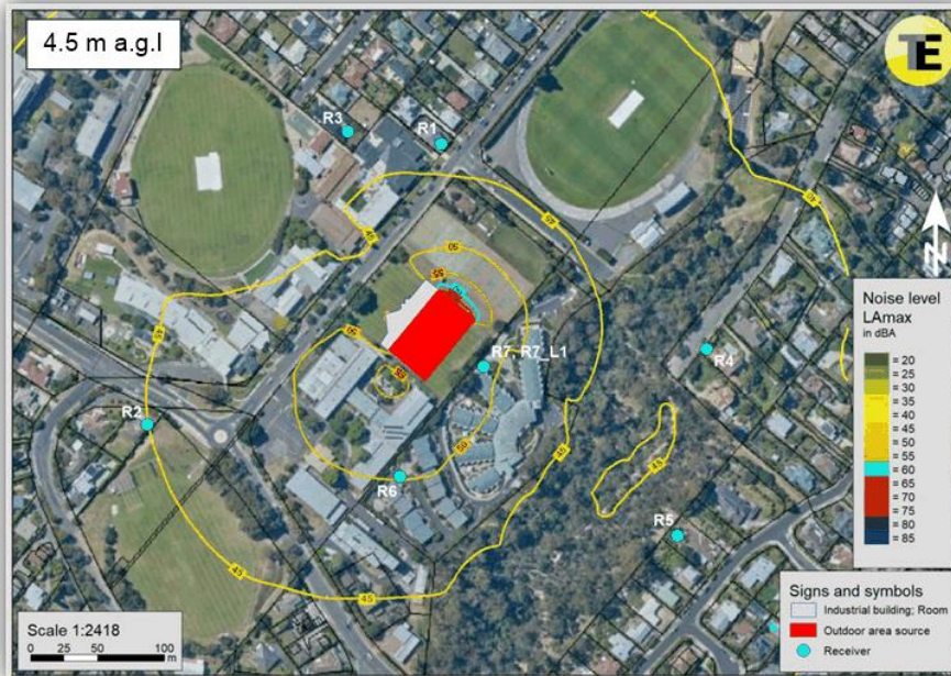
Figure A-4: Predicted noise emission contours, siren and ball impact noise , L_{Amax} , level 1.
