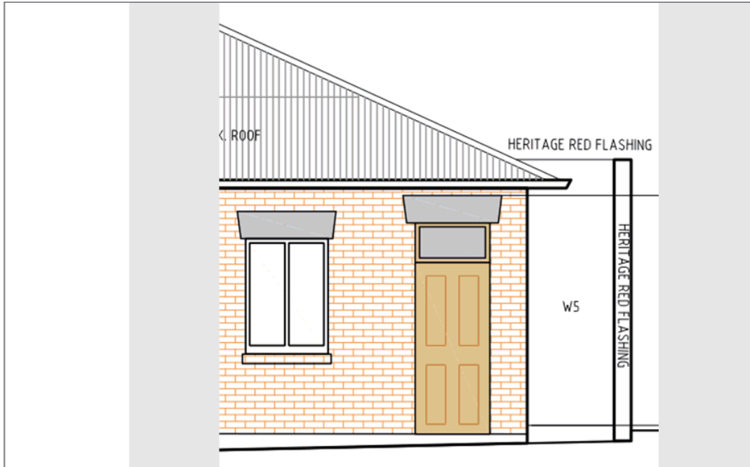
Figure 6: Extract of the proposed western elevation showing the difference in height of the existing cottage side boundary wall and the proposed extension boundary wall (labelled with 'heritage red flashing'). Source: Applicant's documentation, Shurman Design, drawing A06, 'Elevations Proposed', 20.10.2025.
