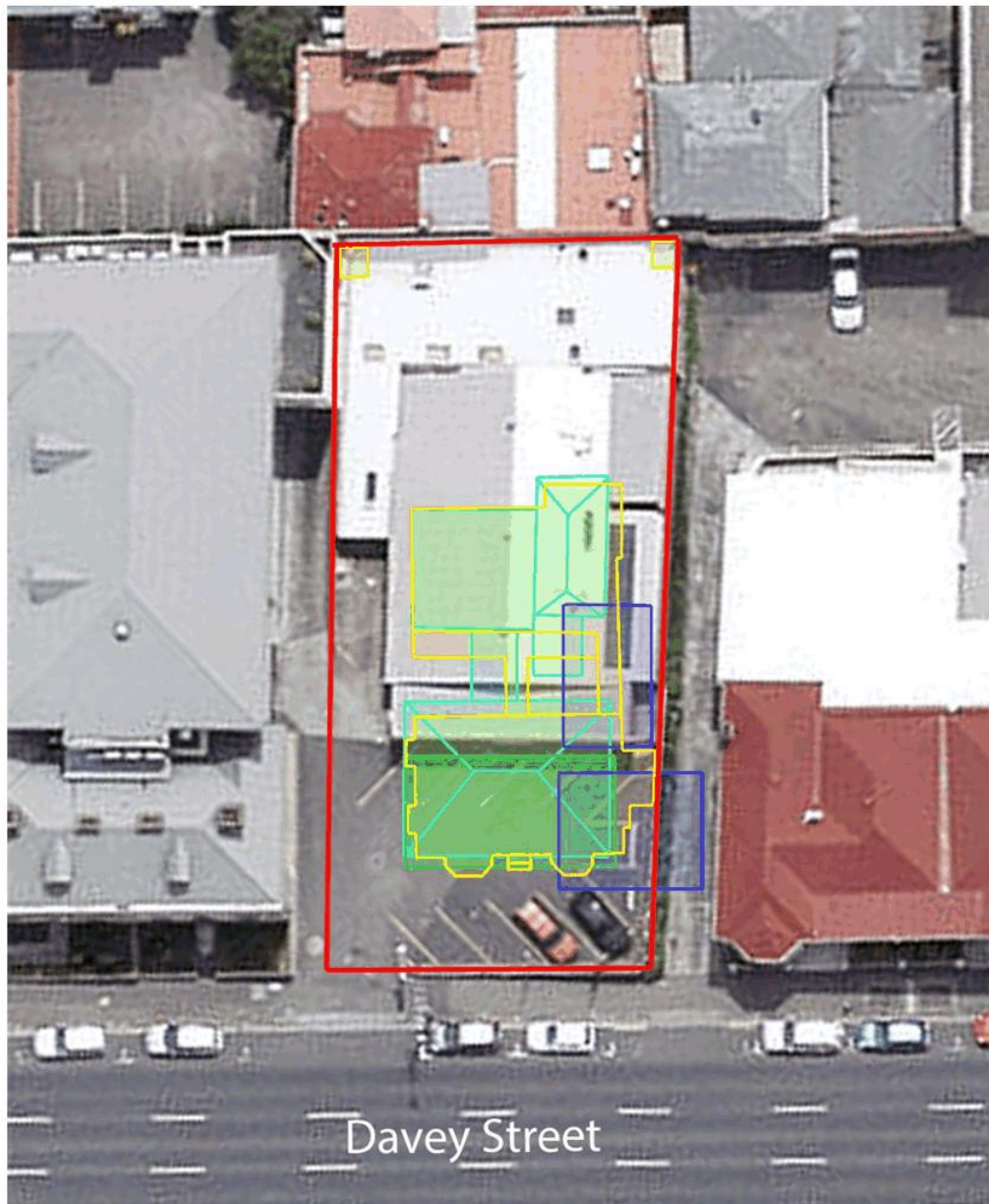
Figure 4.26 – Composite overlay of the footprint of all known pre-1946 buildings and site features (colours as per coding above) in relation to the subject site (red).
