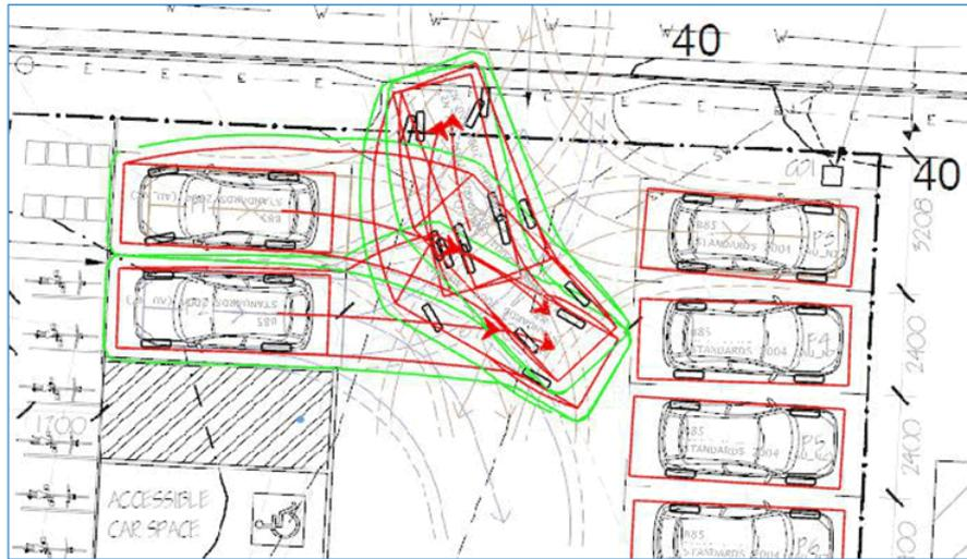
Diagram 4.7D – Swept path of B85 vehicle entering and leaving the accessible parking space
