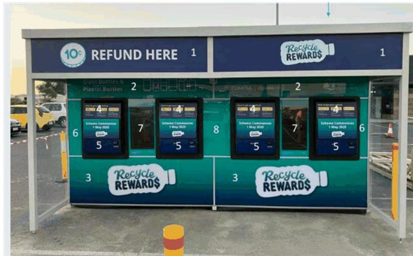
Fig. 6- the front elevation of the container refund machine
