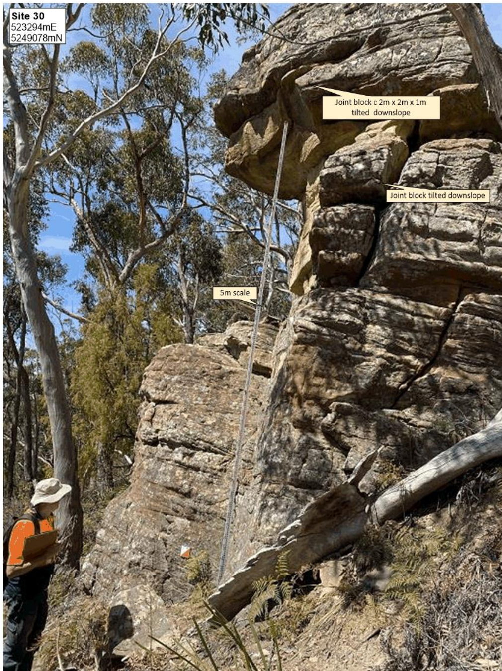
Plate 7. View east across the face of Site 30, a prominent 7m high short cliff section of cross-bedded, strongly-jointed, moderately-highly weathered Triassic sandstone bedrock dipping approx. 10° SSE. The site is about 40m upslope from the proposed track, which in this area follows the existing Pipeline Track. Some joint blocks are overhanging and rotated downslope, and there are several examples of relatively recent rockfalls (up to c.0.5m diameter) at its base and on the slope down to the track.
