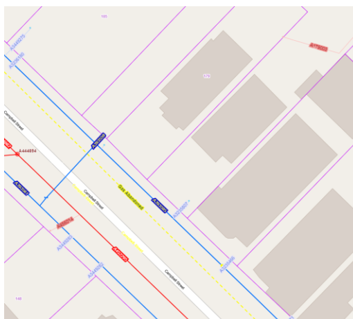
Figure 14: Existing Abandoned Gas Pipe Locations
