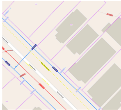
Figure 14: Existing Abandoned Gas Pipe Locations
