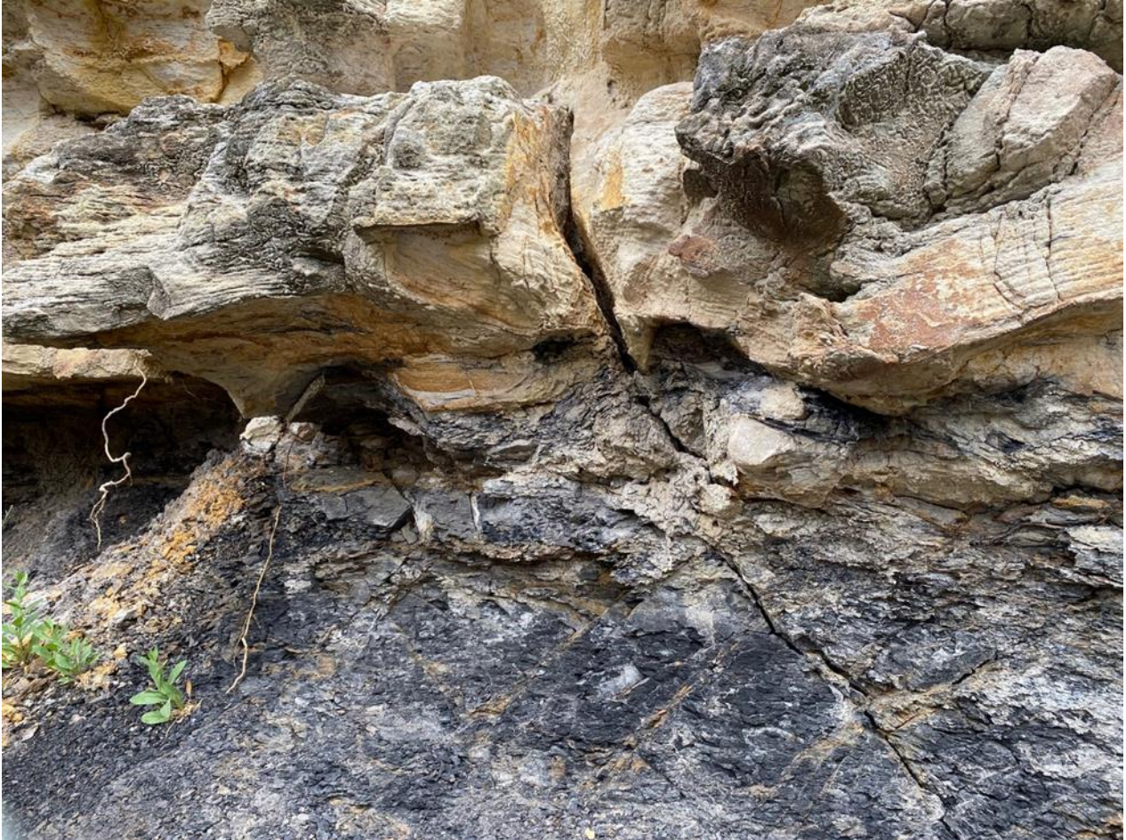
Figure 4. Highly weathered outcrop of New Town Coal Measure, located on the South-eastern side of the site
