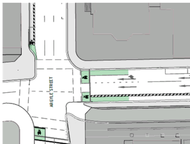
Figure 4 Design drawing for Liverpool Street at Argyle Street
