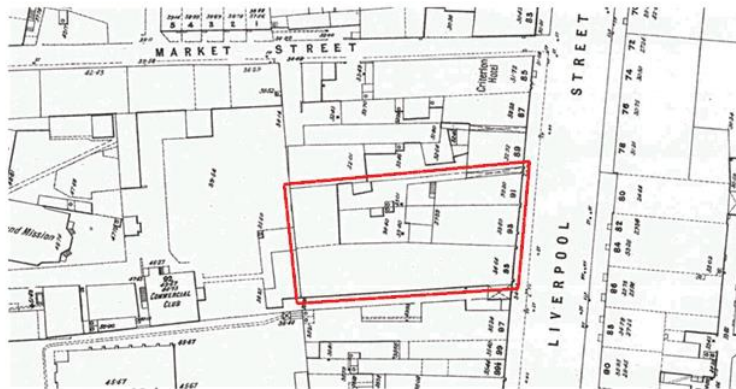
Figure 2: Metropolitan Drainage Plan c.1900 (Tasmanian Archives and Heritage Office). The plan indicates a full depth of building to the south and part depth construction to the middle and northern blocks, a passage to the north, structures to the western boundary and earth closets and other outbuildings in the yards.
