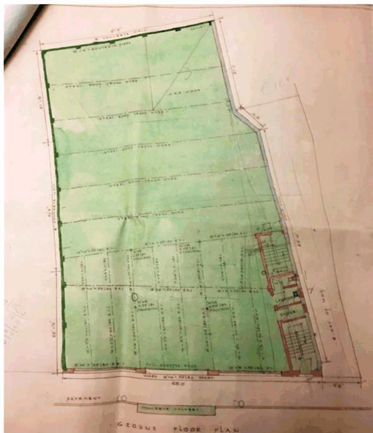
Figure 13: Ground floor plan. The green area shows the building footprint, and area of excavation. The right of way on the north eastern side is indicated (TAHO, AE417/1/2108, 125 Bathurst Street (6871).
