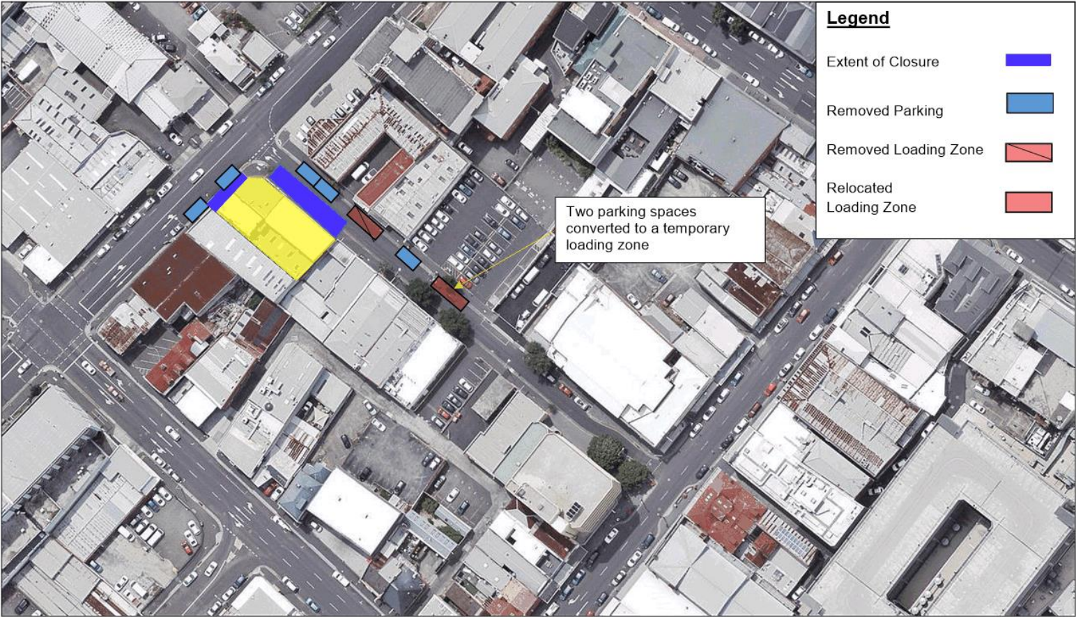
Figure 7 Half Road Closure – Parking Arrangements
