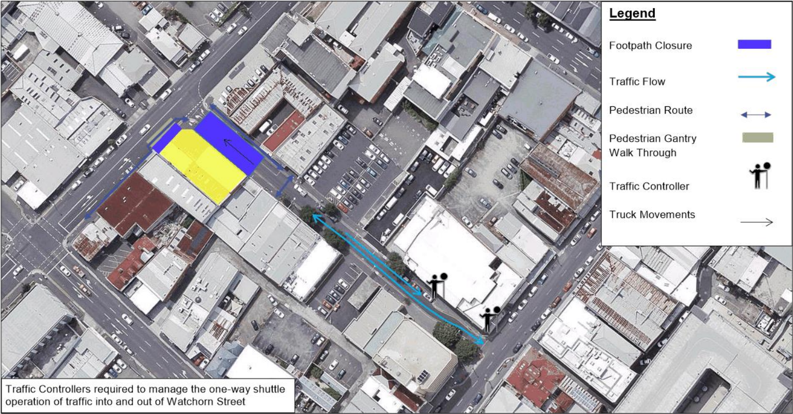
Figure 5 Full Road Closure – Construction Footprint
