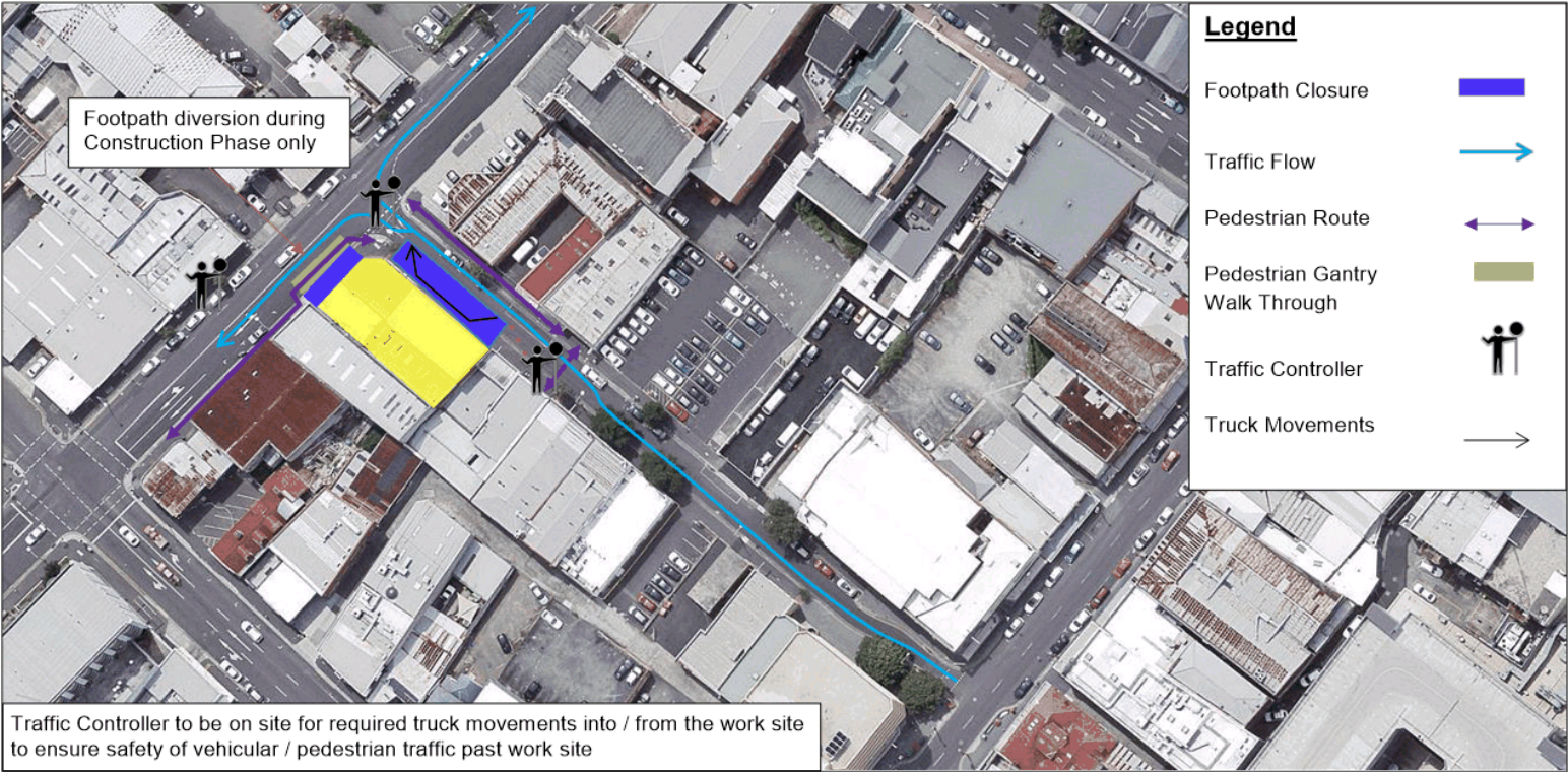
Figure 4 Half Road Closure – Construction and Demolition Footprint
