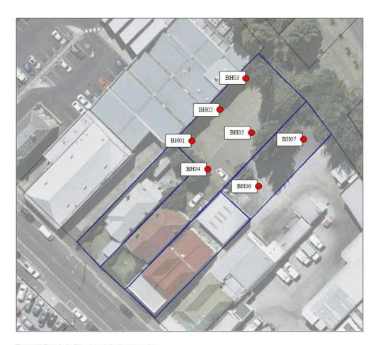
Figure 8 Borehole Plan (Aerial photo overlay)
