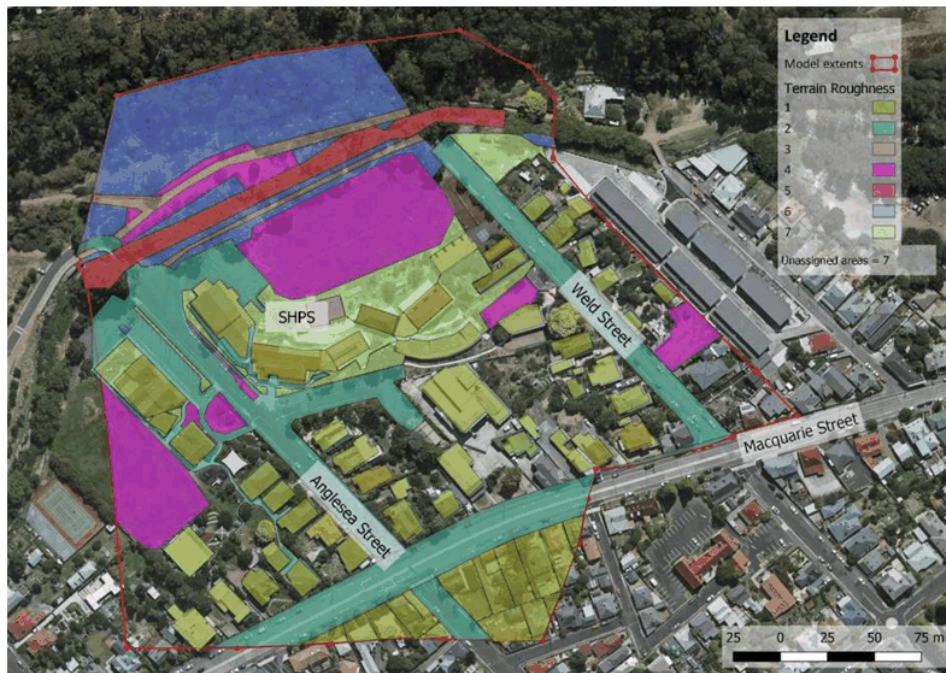
Figure 5.2: Schematic of terrain roughness values
