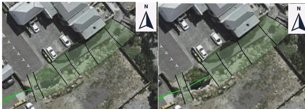
Figure 7: One-dimensional representation of rivulet through site (existing (left), proposed right))
