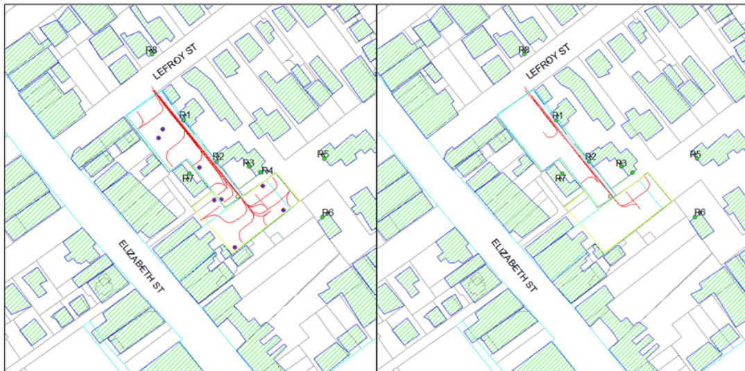
Figure 6: SoundPLAN noise model plan views, Left: daytime scenario, Right: night time scenario
