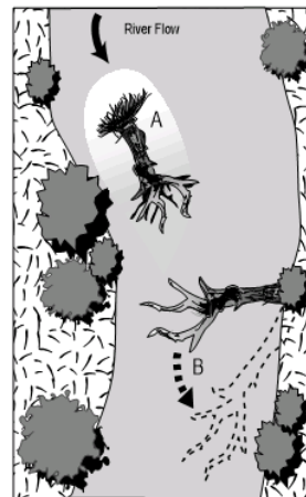
LWD provides feeding and refuge areas for fish and other aquatic species. Hydraulic forces around LWD contribute structural diversity to the river bed - eg upstream scour pools (A). LWD should not be disturbed unless it is shown to be causing unacceptable flooding or erosion. If action is required, re-aligning LWD nearer to the bank is preferred to removal (B).
