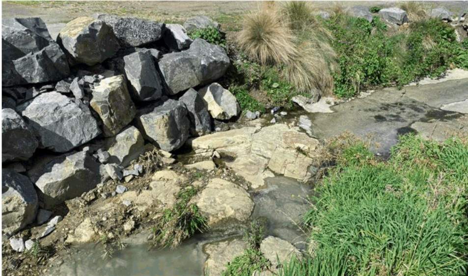
Figure 3: Outcrop of massive sandstone observed at Providence Rivulet Creek bed (Source: pitt&sherry, 2021)
