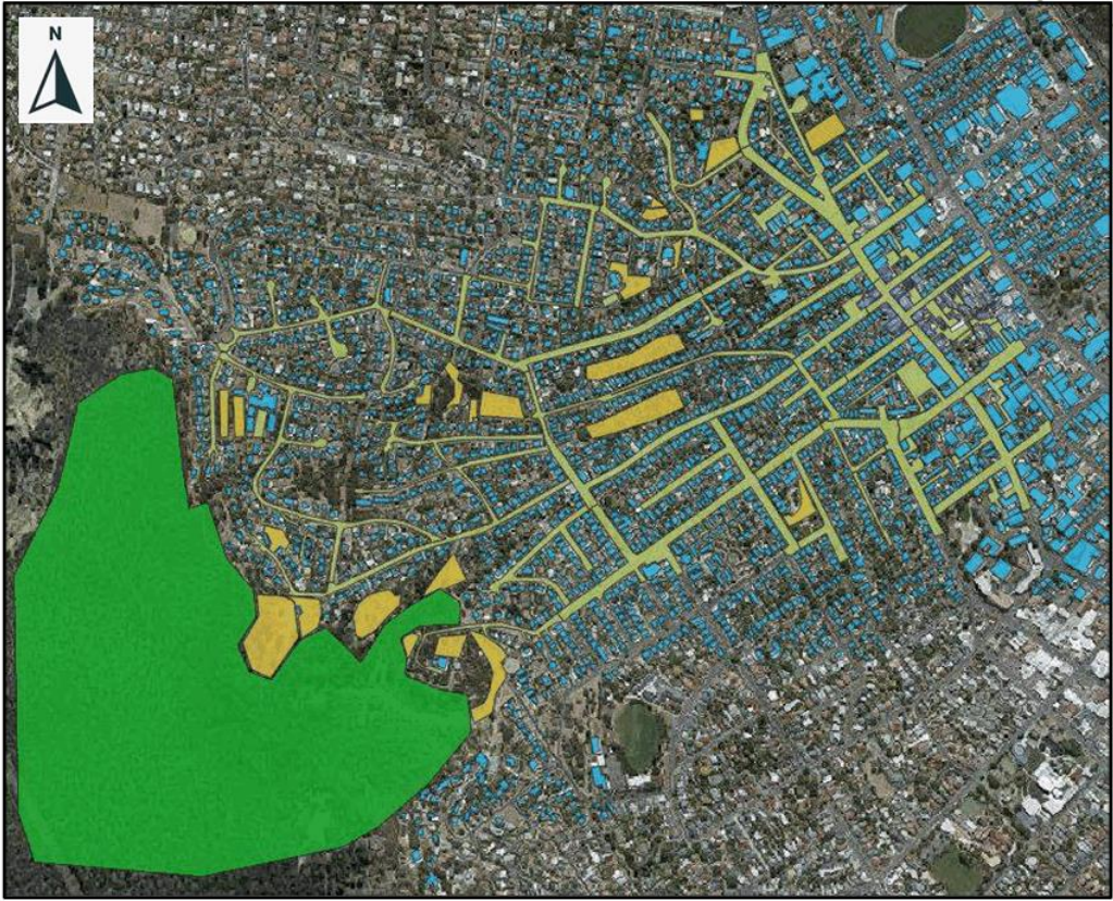
Figure 6: TUFLOW model material roughness layers
