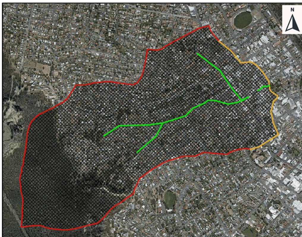
Figure 3: Two-dimensional rain on grid model extents (red), pipe mains (green), downstream boundary (yellow)
