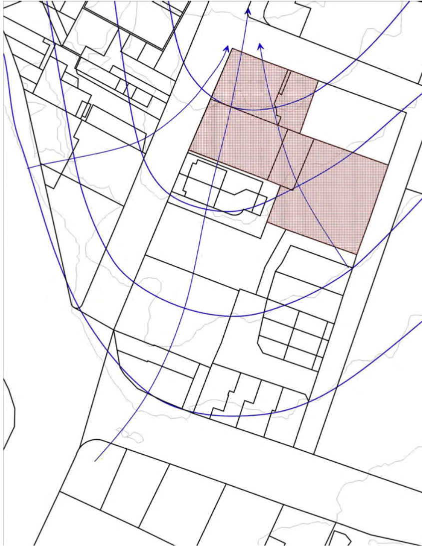
Figure 5: Inferred groundwater flow direction and locations of monitoring wells
