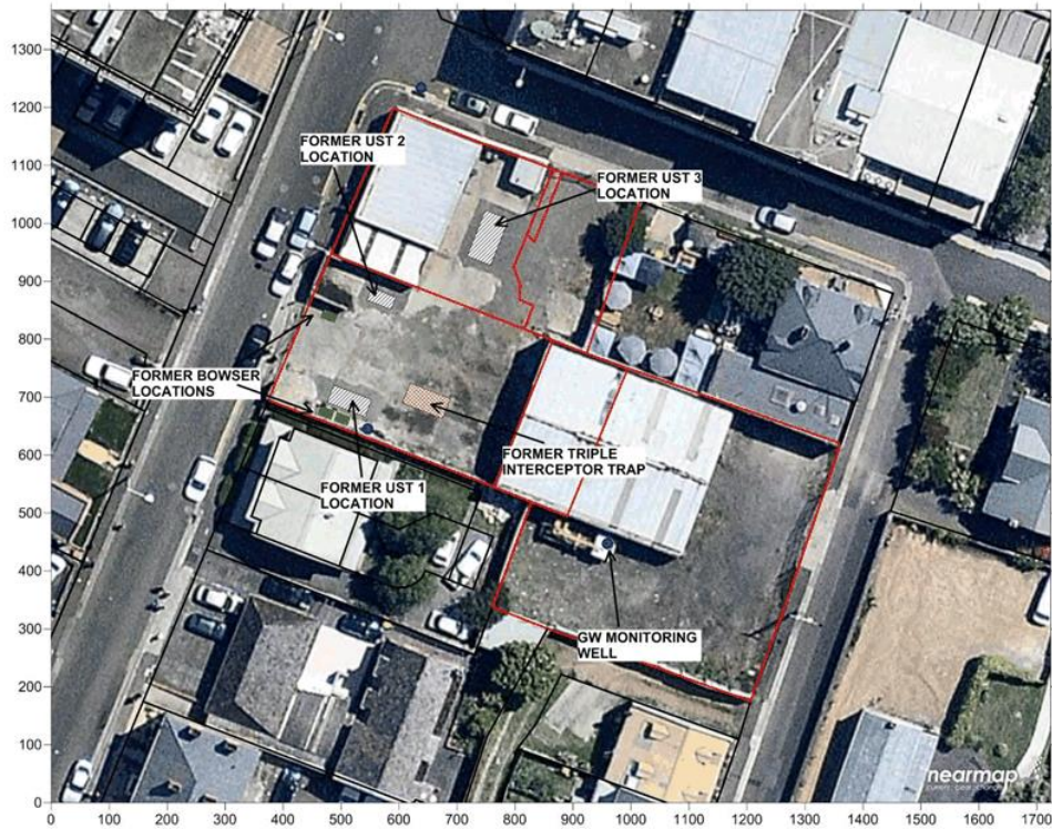
Figure 2 -Aerial photo showing the location of former infrastructure including USTs, bowser locations, triple interceptor trap plus the groundwater monitoring wells.
