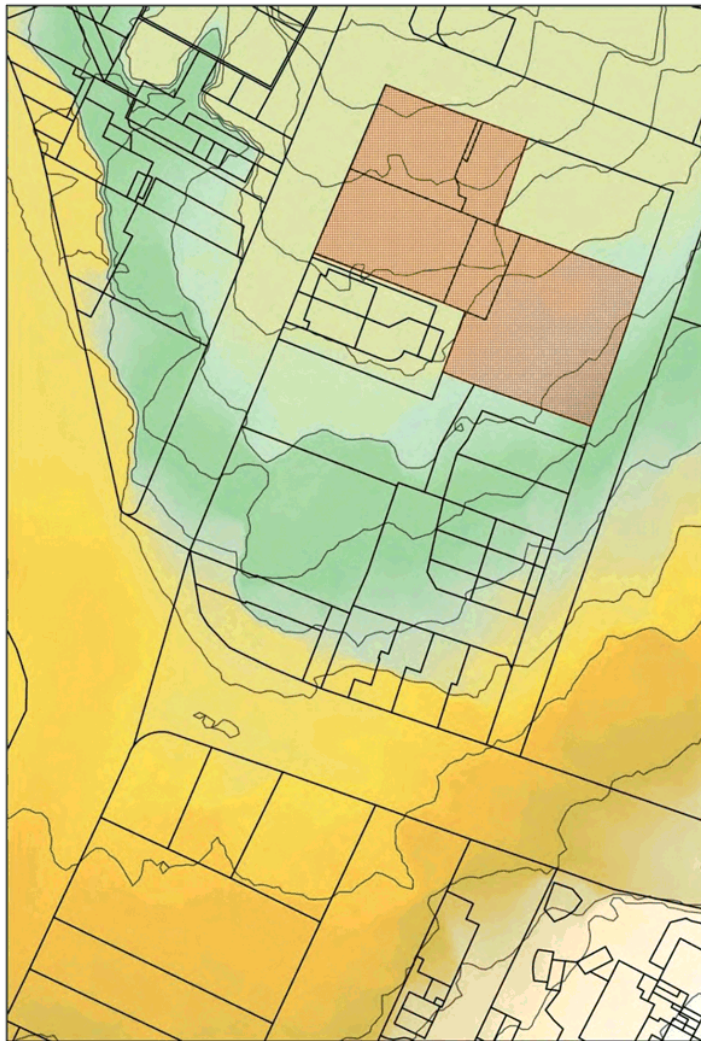
Figure 3: Topography of the site showing LIDAR ground contours at 1m intervals.
