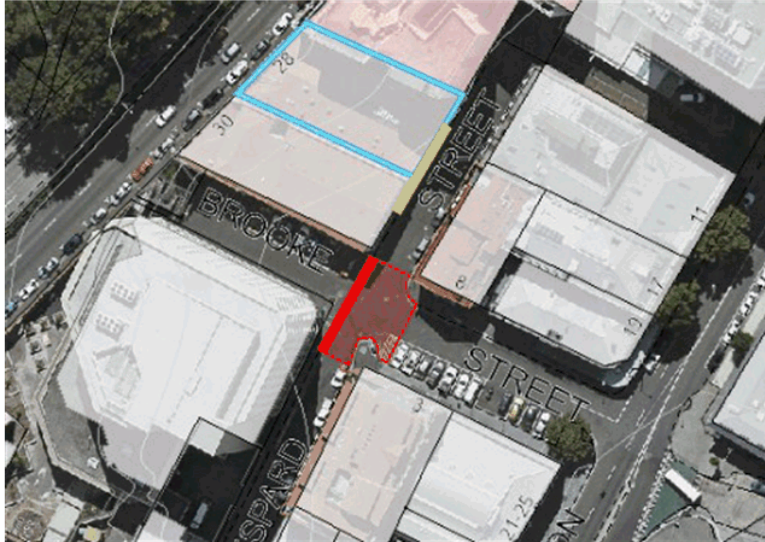
Figure 2: The thick red line and shaded area show the 'kerbless' crossover and New Transition Zone, which is virtually within the vehicle circulation network previously seen in Figure 1. The thick yellow line identifies the length of the proposed crossover, shown to be consuming a significant portion of the existing footpath.
