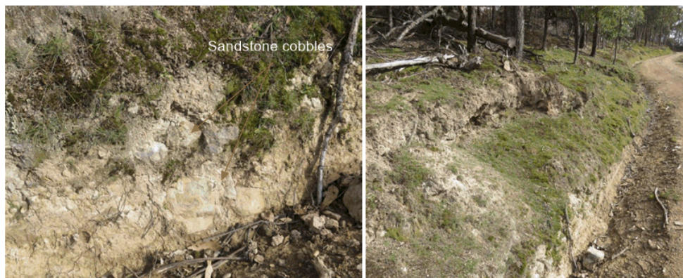
Figure 4-2 Colluvium soil profile exposed in cutting at upslope side of Base Site
