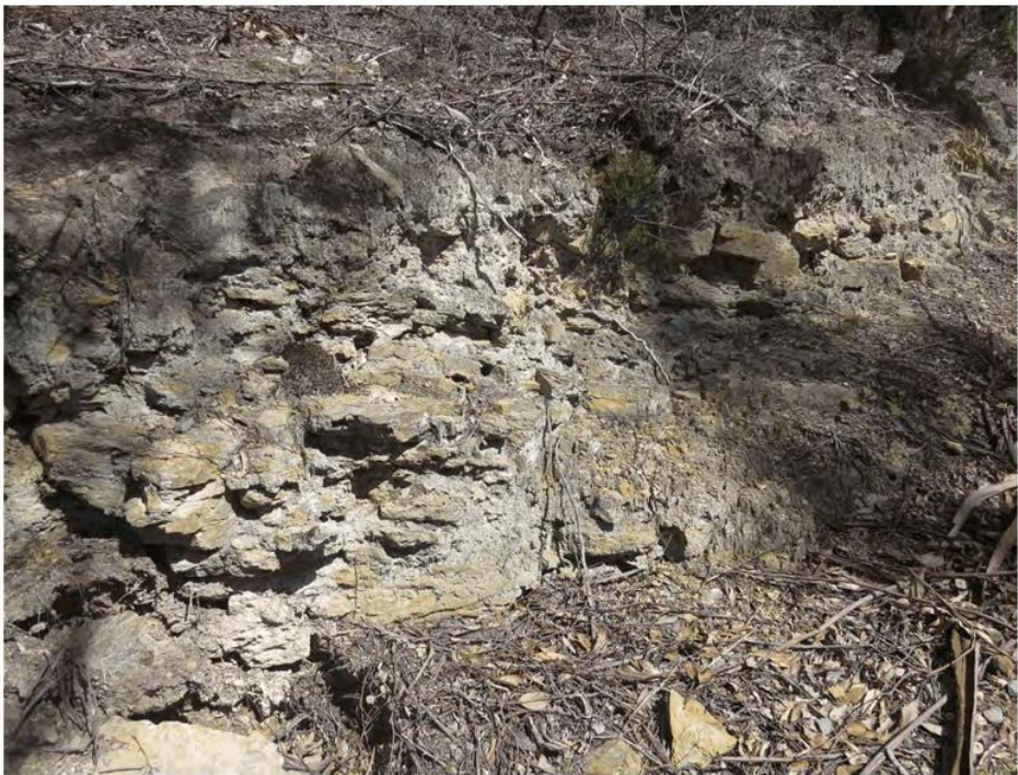
Photo 23 - Extremely weathered Siltstone underlying colluvium exposed in cutting north of base site
