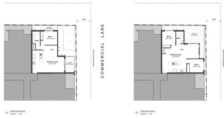
Figure 4: Floor plan of the approved layout on the left hand side, and the proposed layout on the right hand side.
