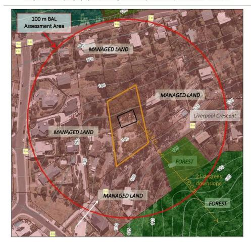
Figure 2 – 100m radius BAL Assessment area showing surrounding vegetation, slopes and direction of photos from the site of the proposed dwelling, refer to Appendix 3 for photos (Image source: LISTmap
