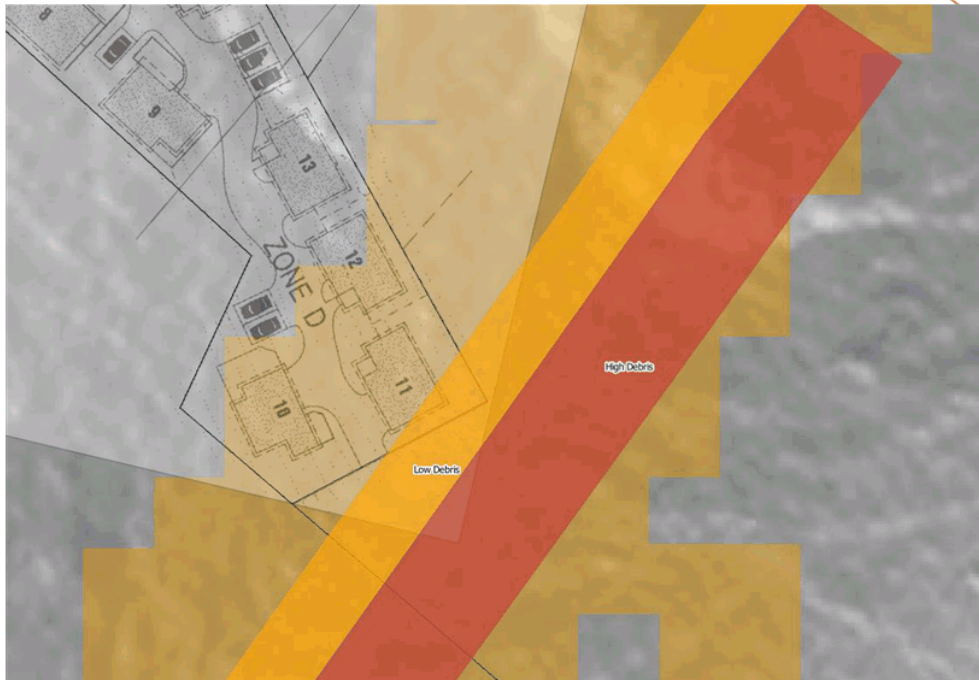
Figure 9: Areas of low debris to west of creek line, high debris to east; hazard band shown
