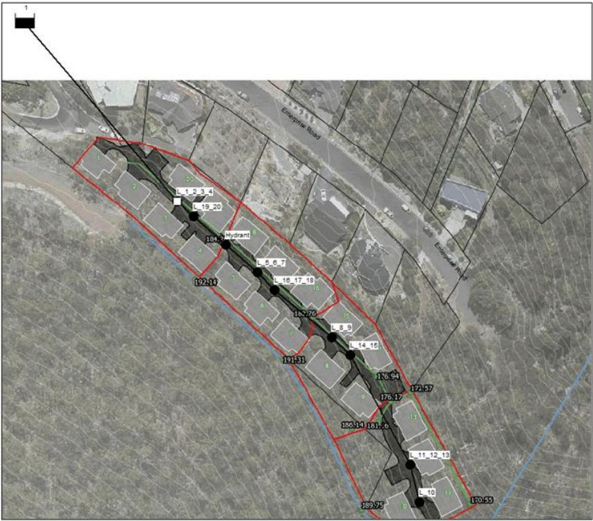
Figure 3: EPANET model layout
