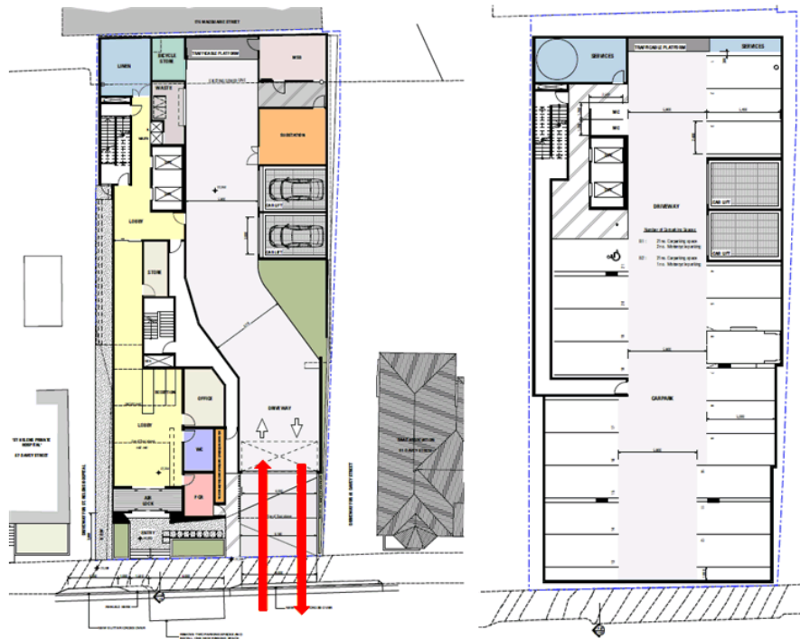
Figure 20: Ground level plan (left) illustrating two-way access and exit to the development from Davey Street. This vehicular access provides routes to an internal car lift, with two levels of basement parking as illustrated in basement plan (right). Source: JAWS Architects.
