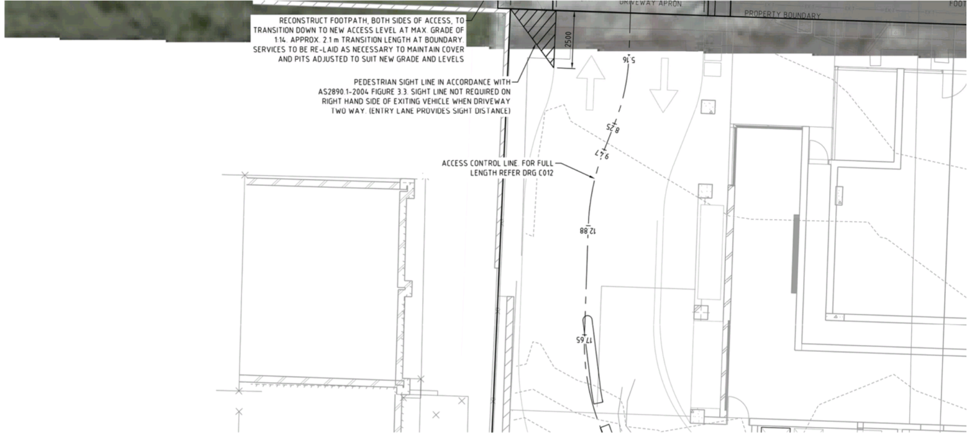
SITWORKS PLAN SCALE 1:100
