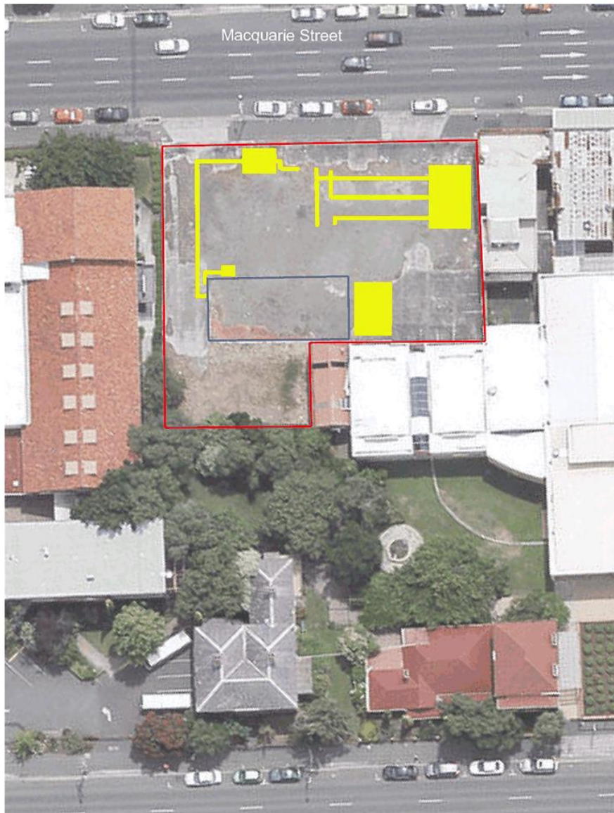
Figure 5.4 – Tank and fuel line locations (yellow) derived from the various environmental reports and historical data (the service station building footprint depicted in blue. Adapted from www.thelist.tas.gov.au
