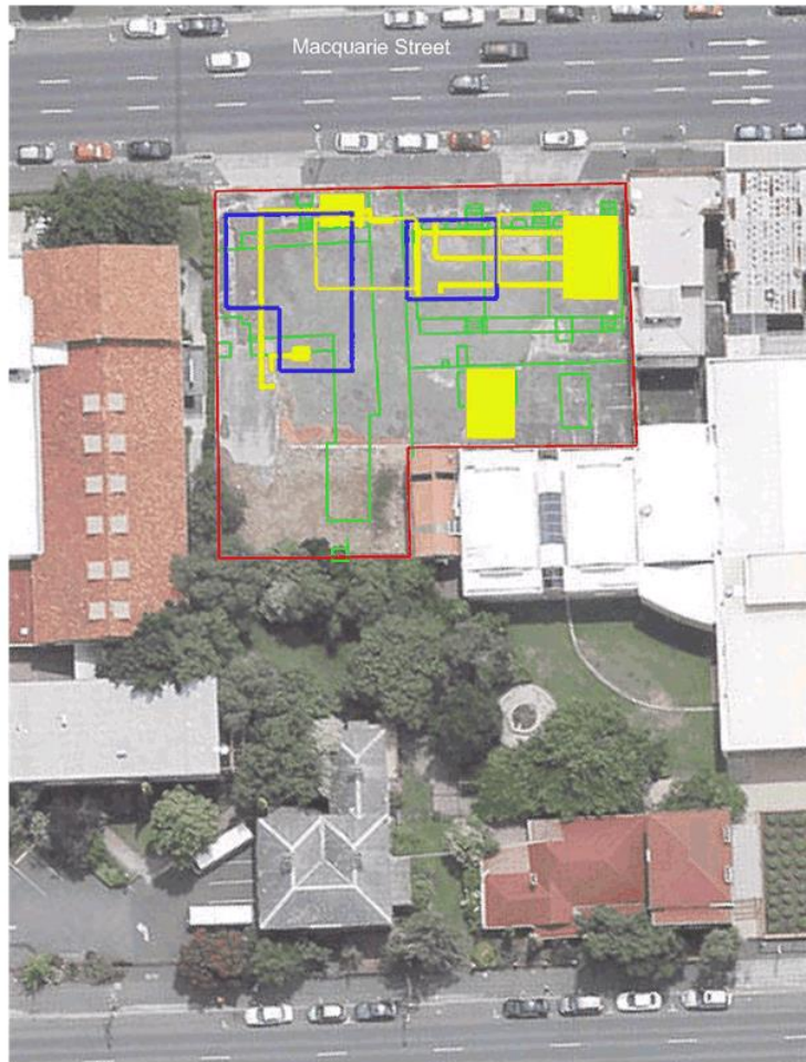
Figure 5.5 – Tank and fuel line locations (yellow) overlaid on historic building footprints (blue = c1832, green = c1850+). Adapted from www.thelist.tas.gov.au
