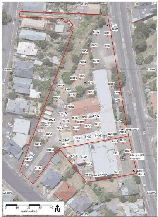
Note: BH#-Soil bores; MW# - groundwater bore and GT# - Geotechnical Hole
