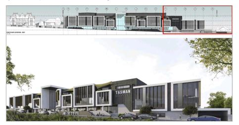
Figure 11: Revised building height and setback along the northern and north-eastern elevation (source:
