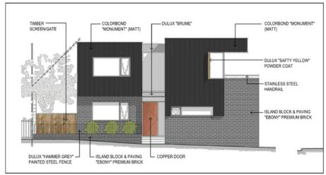
Figure 3: The proposed George Street elevation.
