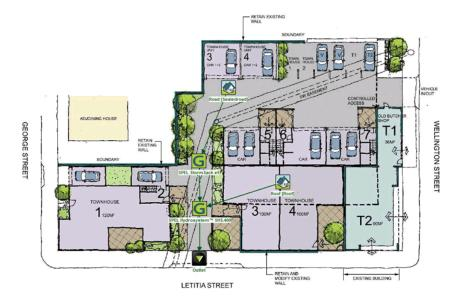
Figure 8 Location of proposed Stormwater Quality Devices
