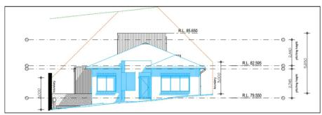
Figure 9: Proposed front elevations. Existing development is shown in blue.
