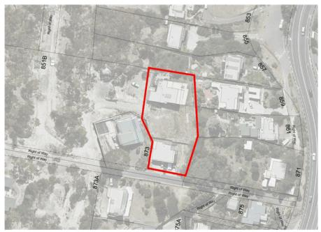
Figure 4: Location of the approved dwellings is generally indicated by the red border. Only two of the three dwellings have been constructed. The approval stipulated that only the bottom (southern) dwelling was allowed to gain access via the driveway that is the subject of this planning application. The other two houses were to be accessed via the right of way to the north over 851A Sandy Bay Road.
