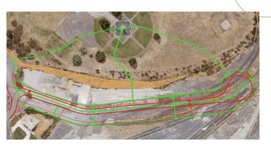
Figure 3 Catchment Plan (catchments in green), 0.2m contour spacing (orange)
