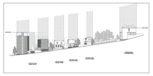
Figure 17: Elevation plan showing the variable heights of buildings along Wilmot Street in response to the topography (source: Room 11 Architects)
