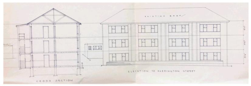
Figure 2.21 - Proposed elevation and section of the conversion of Wilmot Terrace. The four bays of the original houses are discernible on the elevation.
