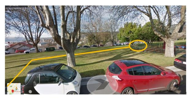
Fig 1: Approximate location of the new kiosk substation and the new cabling within the park
