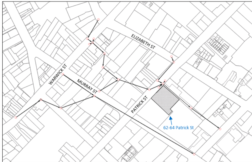
Figure 5. XPSTORM modelled underground pipe network.
