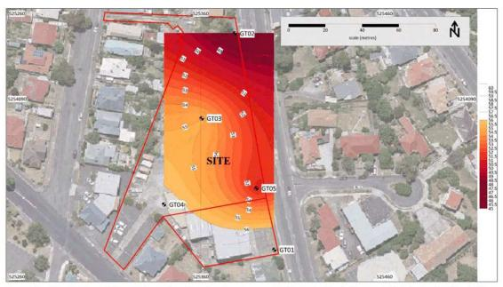
Figure 4 Elevation of the base of fill material encountered (area in read and orange and red indicates fill underlying expected design level of 55.8 m AHD) (Coordinate System: GDA94 MGA Zone 55)
