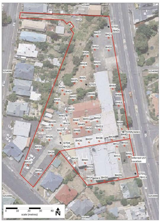
Figure 10 Borehole Plan
