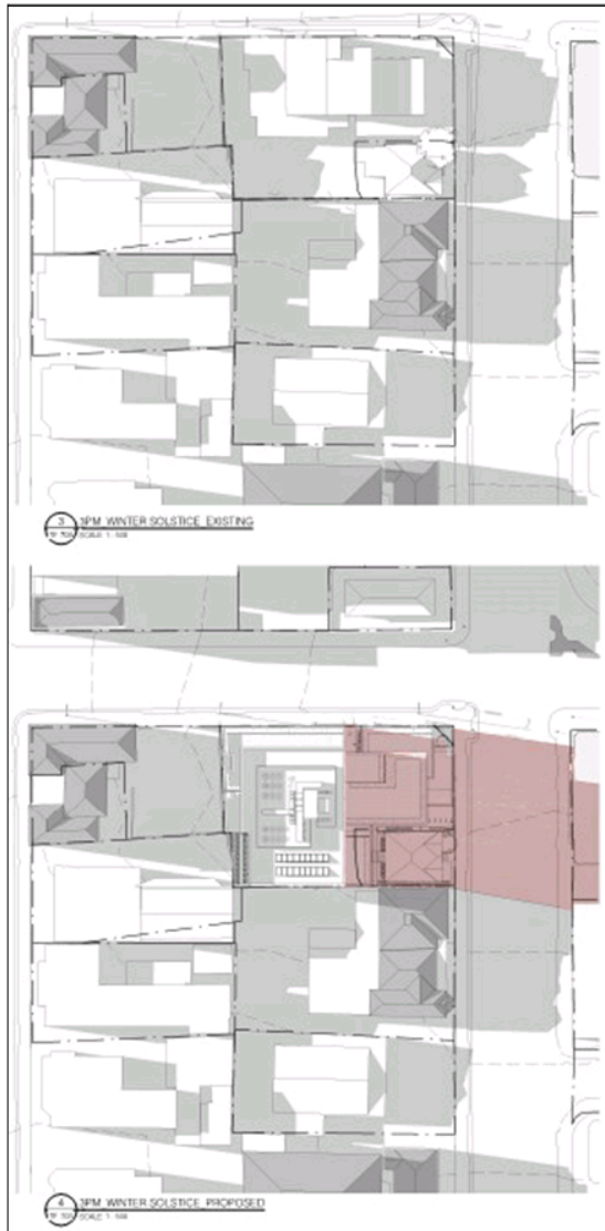
Figure 13: Shadow Study, 3pm on winter solstice - proposed impact shown in red, existing impacts in grey (provided by applicant).
