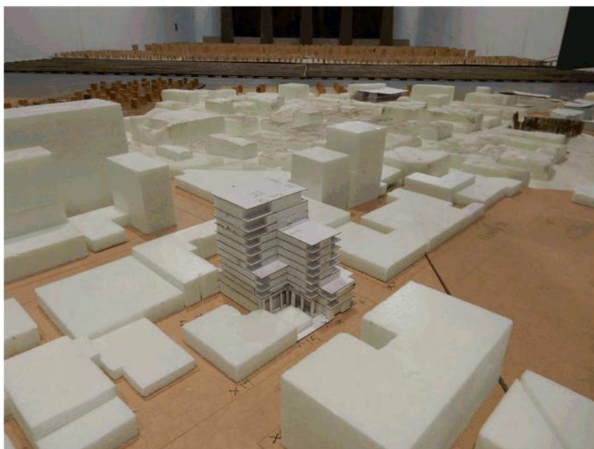
Figure 4 – Close up view from the south of the 1/400 scale model of the 58 Harrington Street Development in the wind tunnel.
