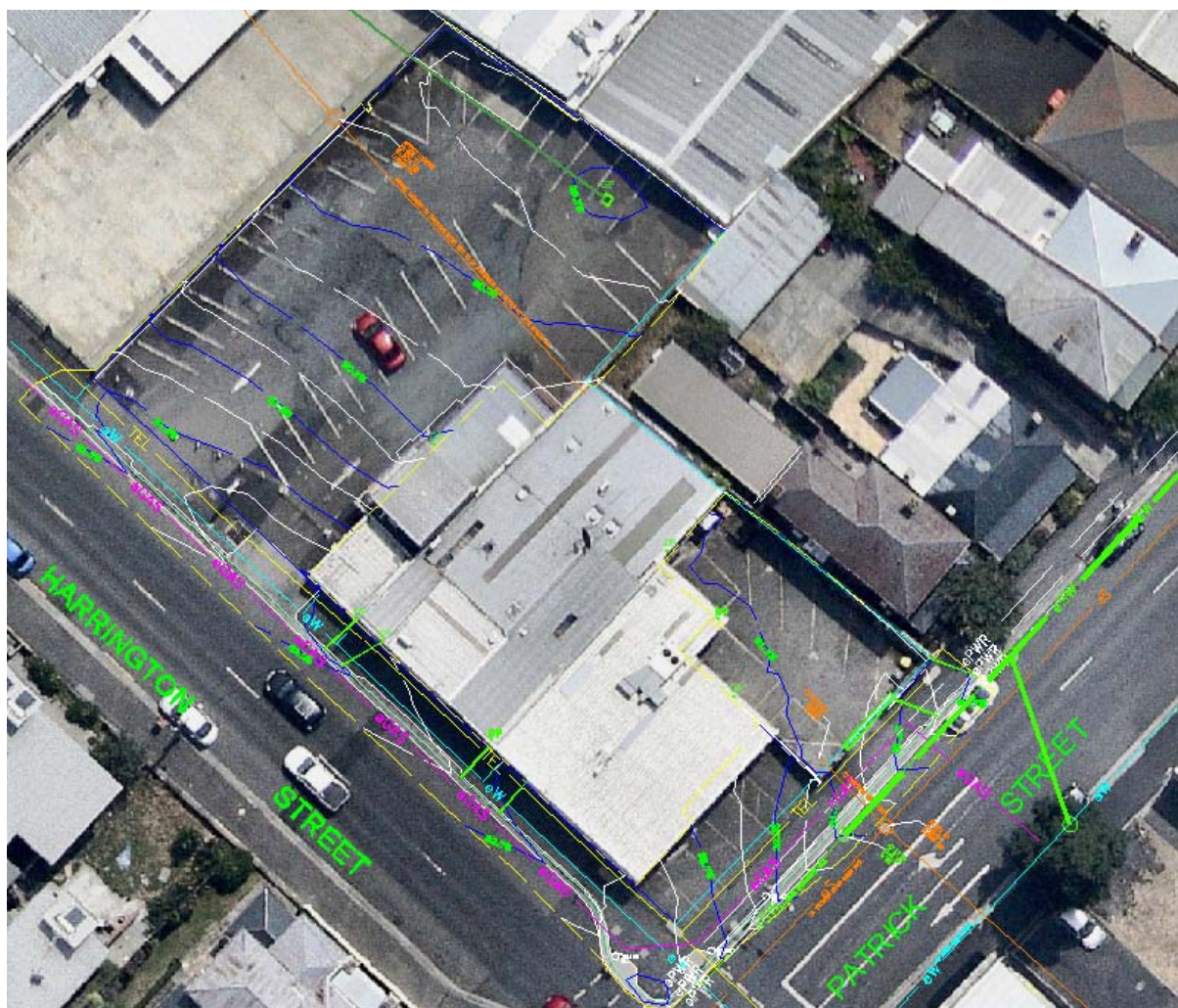
Figure 2 - site plan showing existing services.
