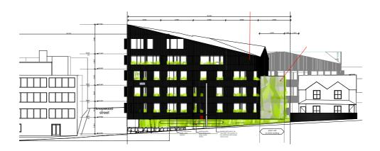
There is an existing building on the corner of Knopwood and Montpelier, which we understand may be reasonably old, has been very badly altered, to a point where there is now negligible value in the structure, but the foundation plinth is sandstone whereas the upper walls were brick, now rendered. We intend to retain the stone plinth and use it as part of creating a link with history at street level.
