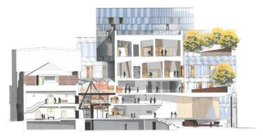
Figure 23: Collins Street entry section - Showing corner glazed entry 'box' and stairs up to the principal foyer levels with glass roof over and connection to TR foyers.
