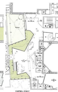
Figure 35: Foyer floor plan - Level 4 Lobby and bar highlighting voids (in green) abutting the TR heritage Wall,
