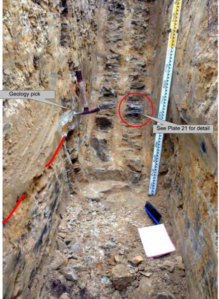
Plate 20 (left). Investigation trench B, upslope end, showing finely bedded, highly weathered sandstone and siltstone bedrock dipping 3<sup>0</sup> to 017<sup>0</sup>T. Colluvium (with some bedded sandstone) overlies the bedrock, and the boundary (red line) between them, not although very obvious, is inferred to dip towards and up to the camera in a scallop shape (the geology pick on is boundary).
