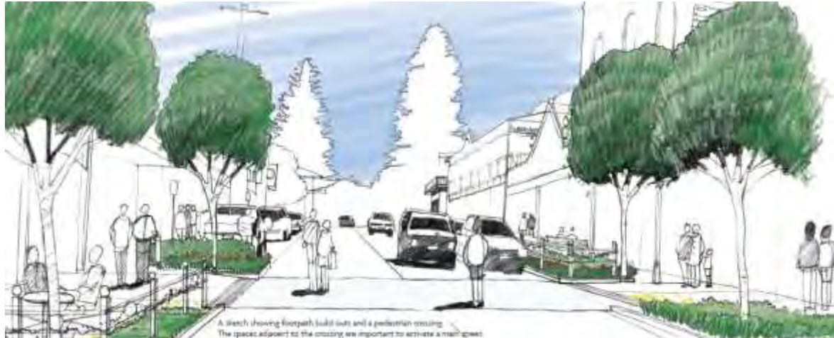
Figure 3.4: Pedestrian crossing build out with median refuge
